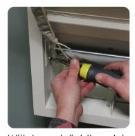
With board slightly out, install the screw in the bottom hole on left side pivot plate. Then, raise the board back into cabinet and use retainer bar to hold in place.
