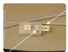
Top Prong (Connect wire from unit) Bottom Prong (Connect wire from timer)
